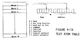
The Text Atom table occupies 96 entries in the 8-bit ROM (see Figure 4-16). Each entry consists of a 16-bit pointer for every possible text atom. When an atom is requested, two bytes of 8-bit ROM are read from the Text Atom table at the address of the entry number specified by the atom.
