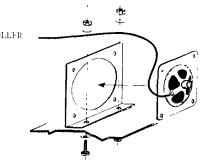
(d) Rcute speaker cable out via CRT cable hole in 2216 or 2220 chassis and plug this cable into the 2216/2220 CRT controller board (6312A) or 6350A).
