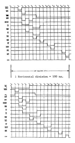
FIGURE 4-13 MODEL 2200 S/T CPU TIMING
