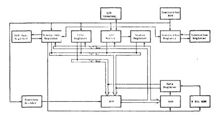
FIGURE 4-1 SIMPLIFIED 2200 CPU BLOCK DIAGRAM
