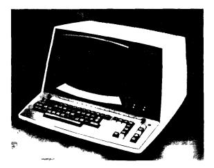
A Video Display Controller (located in a CPU I/O Slot) is used to control display of dot matrix characters on a Cathode Ray Tube screen (CRT) by providing video information and all required synchronization/ timing signals.
