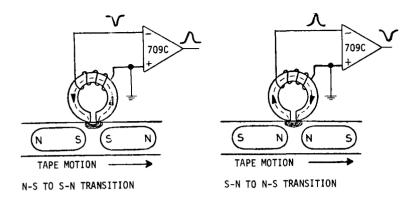
FIGURE 5-18 TAPE DATA SENSING
