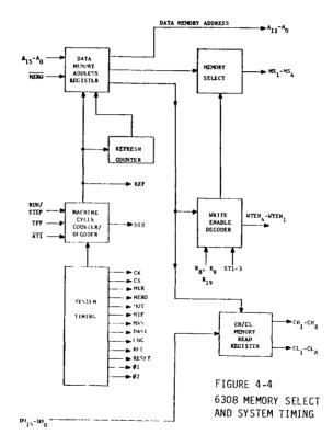
used to address data words in the 8 bit ROM or to address data words being read from or written into the RAM. During RAM Refresh cycles, the Data Memory Address Register receives the RAM column address from the Refresh Counter (6308-L26, 27).
