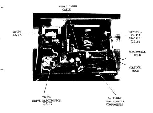
The 2216 Video Display is comprised of an 8" x 10.5" CRT mounted in a Motorola display chassis (Motorola #XM351). Also mounted within the Motorola chassis is the CRT electronics plug-in circuit board (Motorola #V13A).
