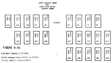
Change labels on 6735 (A, B, or C) and 6708 (A, B, or C) to 6735D and 6708D respectively.
