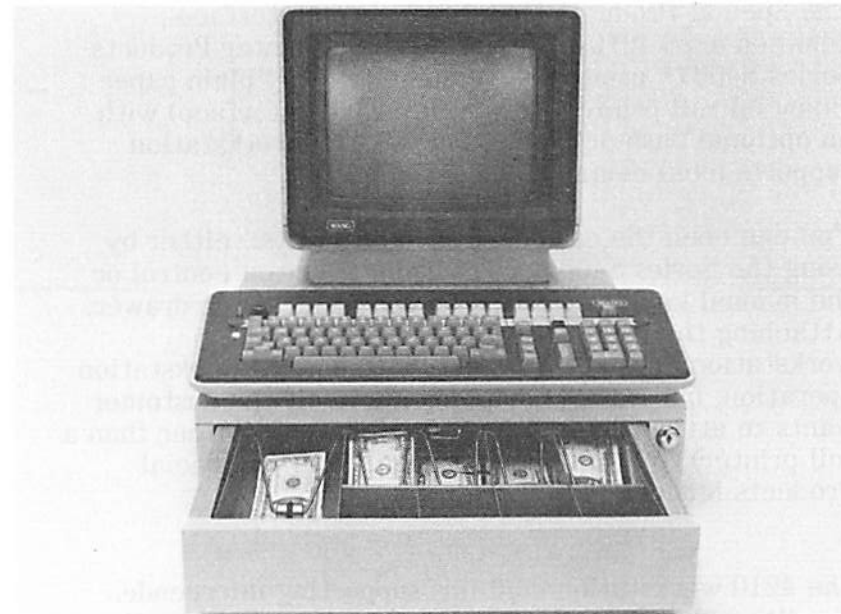
The Model 9129 serves as an interface between an Indiana cash drawer and a 2336 DE/DW workstation.
